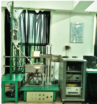
Fig. 2 Photo of the gradient material SLM molding system with a device of real-time mixing powders in various ways
