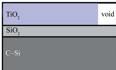
Fig. 2 Model of film structure with voids for ellipsometry fitting
