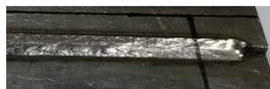
Fig. 4 Surface morphology of weld under full gas protection
