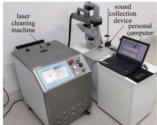
Fig. 1 Device diagram for acoustic monitoring of laser cleaning
