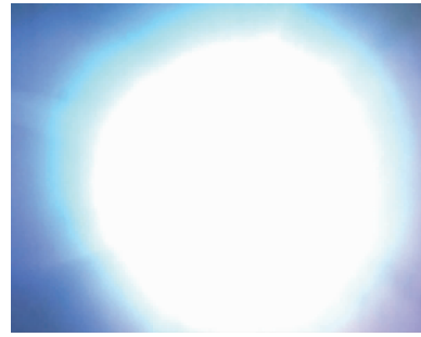
Fig. 14 935 \mu W white light disturbs color CCD image
