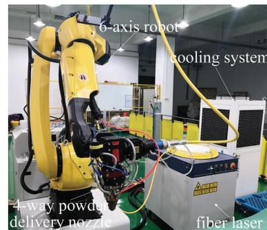
Fig. 2 Testing system of LMD
