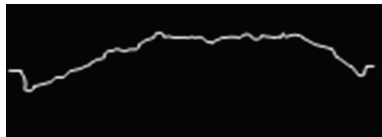
Fig. 7 Extraction result of laser stripe centerline
