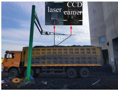
Fig. 9 On-site measurement system construction
