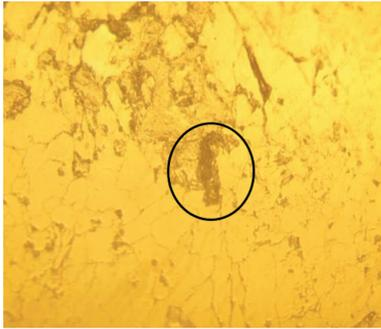
Fig. 4 Photograph of glue injection jade gap under microscope
