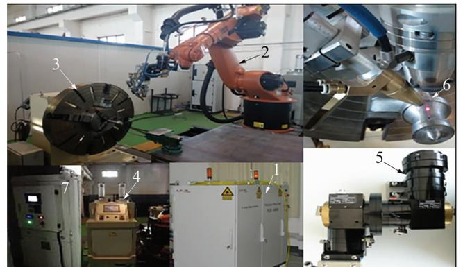
Fig. 1 Laser cladding experiment equipments (1—fiber laser YLS-4000-S2; 2—KR30HA robot; 3—servo rotating worktable; 4—XSL-PF-01A-2 negative pressure type powder feeding system; 5—PLFDH0125 laser head; 6—lateral powder-feed nozzle; 7—cooling system)
