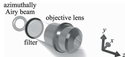
Fig. 1 Schematic setup to generate the super-resolution and transversally polarized light needle
