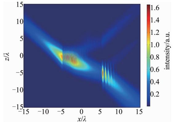
Fig. 4 The normalized internal-field and near-field of a TE mode Gaussian beam through an uniaxial anisotropic cylinder
