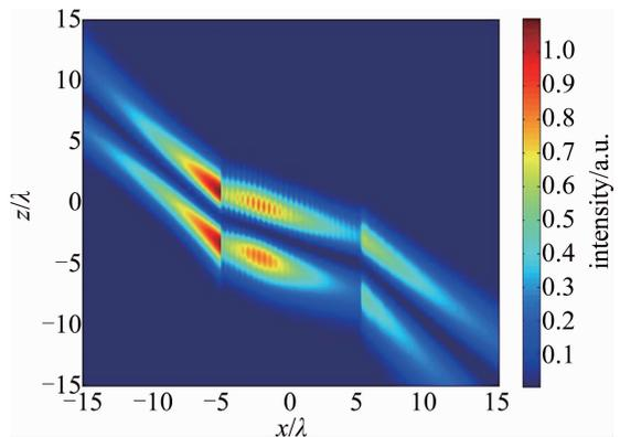
Fig. 5 The normalized internal-field and near-field of a  $TEM_{10}^{(x')}$  mode Hermite-Gaussian beam through an uniaxial anisotropic cylinder
