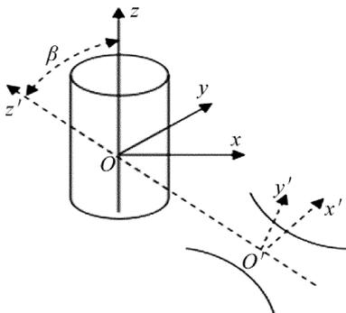
Fig. 1 The incidence of a Gaussian beam on an uniaxial anisotropic cylinder
