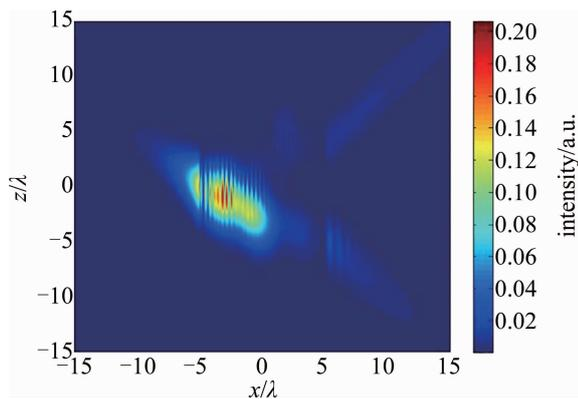
Fig. 6 The normalized internal-field and near-field of a  $TEM_{10}^{(x')}$  mode Hermite-Gaussian beam through an uniaxial anisotropic cylinder
