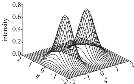
Fig. 3 The intensity distribution of the  $TEM_{10}^{(x')}$  mode Hermite-Gaussian beam
