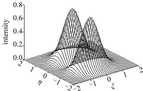
Fig. 2 The intensity distribution of the  $TEM_{10}^{(y')}$  mode Hermite-Gaussian beam
