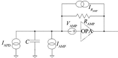
Fig. 4 Noise model of APD detection unit
