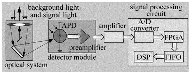
Fig. 1 Block diagram of laser ranging receiving system
