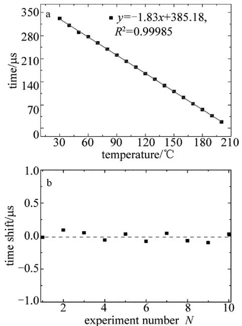
Fig. 8 a—relationship between ring-down time and temperature in experiment
