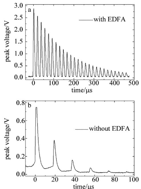
Fig. 5 Ring-down spectrum with and without EDFA
