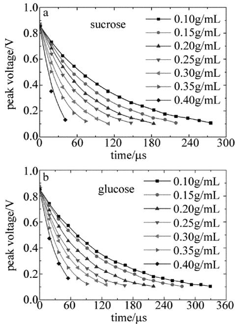
Fig. 6 Fitting curves of ring-down spectrum under different solutions
