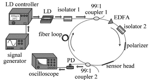
Fig. 1 Experimental setup of based on FLRDS
