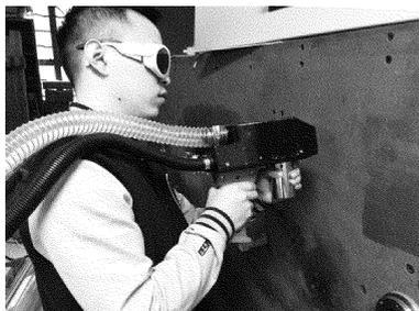
Fig. 4 Hand-held laser scanner of laser cleaning equipment
