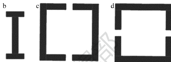
Fig. 2 Transmittance spectrum of light and dark mode and their structures a—transmittance spectrum of light and dark mode b—structure of bright mode c—structure of U-shaped rings as bright mode d—structure of U-shaped rings as dark mode
