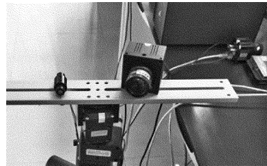
Fig. 4 Experimental device of laser triangulation distance measurement
