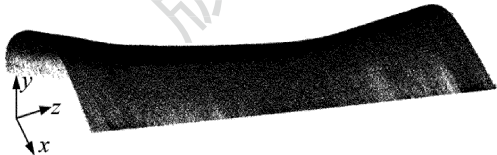
Fig. 2 Cloud data of 3-D profile point of blade trailing edge
