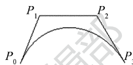
Fig. 2 Cubic Bezier curve
