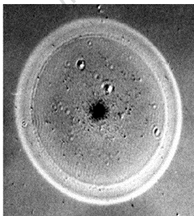
Fig. 2 Nomarski optical micrograph of silicon sample surface treated with single laser pulse in air ( \lambda = 800\text{nm} , \tau = 130\text{fs} , \phi_0 = 1.5\text{J}/\text{cm}^2 )
