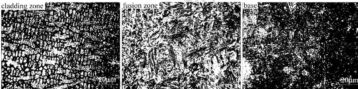
Fig. 10 Microstructure in each region of double-layer and single-channel for cladding material 3540 (500×)
