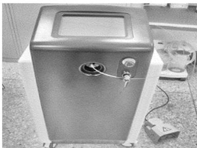
Fig. 3 Prototype of Cr,Tm,Ho:YAG laser lithotripsy system
