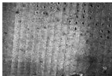
Fig. 5 Microlens array damaged by laser
