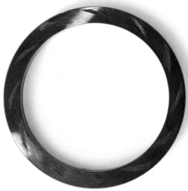
Fig. 6 Planar array applied in mechanical seal ring
