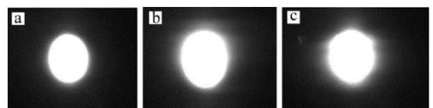
Fig. 3 Laser backscatter images at wavelength of 970nm a—green leaves b—yellow leaves c—dry leaves
