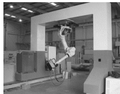
Fig. 1 New equipment of diode laser surface hardening for dies
