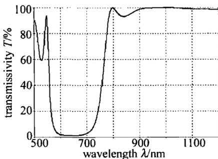
Fig. 2 Transmissivity of spectrum splitting filter film
