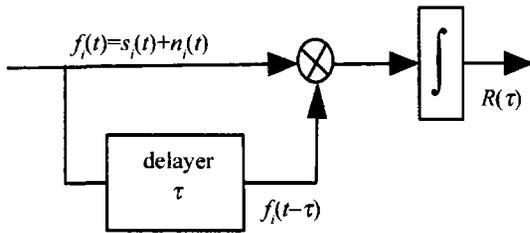
Fig. 4 Block diagram for autocorrelation detection
