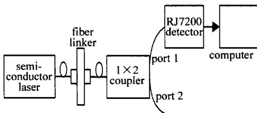
Fig. 6 Sketch map of input optical power testing
