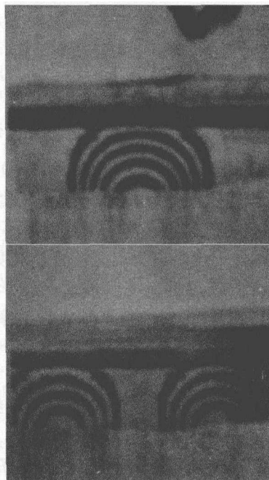
Fig. 4 The interference patterns of 1 \times 2 Y-branching \text{Tl}^+ - \text{Na}^+ ion-exchange waveguide
