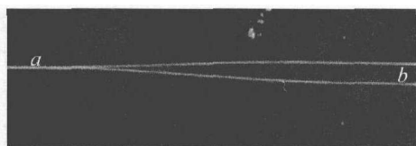
Fig. 3 1 \times 2 Y-branch optical waveguide formed by \text{Tl}^+ - \text{Na}^+ ion exchange
