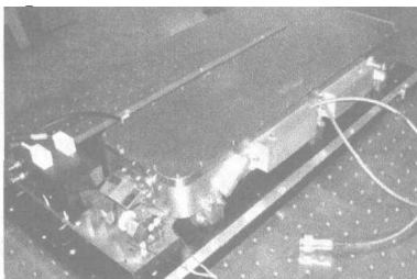
Fig. 2 The waveguide CO 2 laser head
