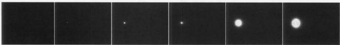
Fig. 4 Laser spot images under variant intensity illuminating ( 0.01 \mu\text{J}/\text{cm}^2 \sim 5.16 \mu\text{J}/\text{cm}^2 )
