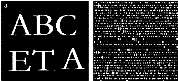
Fig 1 a—original object b—complex matched filter fabricated by CGH
