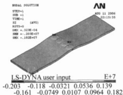
Fig 4 Sheet deformation after implicit static analyse
