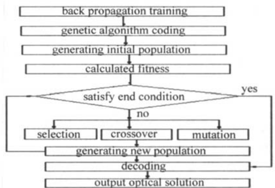
Fig 2 Flow chart of ANN-genetic algorithm combined optimization structure
