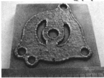
Fig 2 Metallic part of laser freeform fabrication
