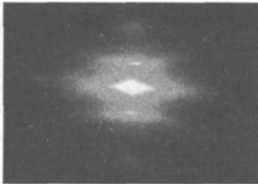
Fig 2 The distribution of light transmitted from chicken muscle tissue at far field
