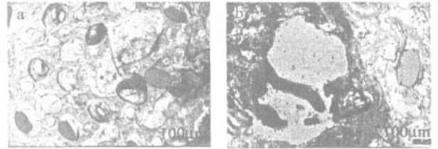
Fig 3 Damaged pattern of the thin film on the surface of a special component dynamic is 0.4^\circ/\text{s} , irradiation time is 5s a— 148\text{W}/\text{cm}^2 , damage diameter is 3.8mm b— 248\text{W}/\text{cm}^2 , damage diameter is 5.5mm
