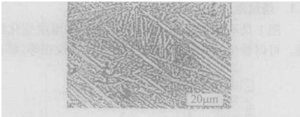
Fig 3 Typical martensite micrographs of a \text{Cu}_{75}\text{Al}_{25} sample
