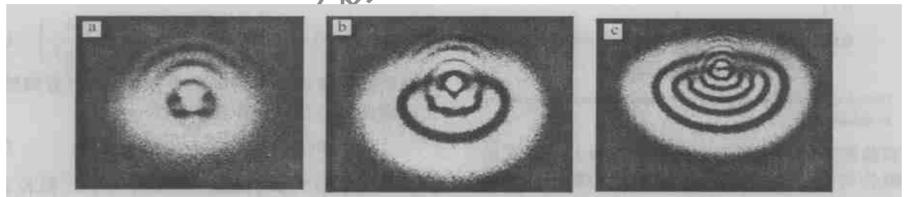
Fig.4 Diffraction rings induced by dominant thermal optic effect
