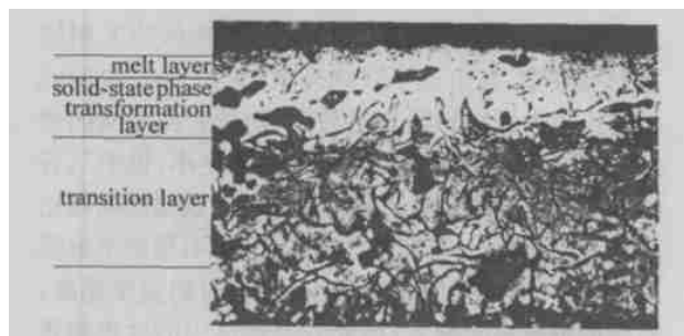
Fig. 1 Micro-structure of laser hardening layer of gray iron 400 ×
