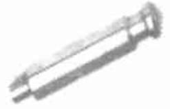
Fig. 4 The exterior of punch pin after laser beam hardening
