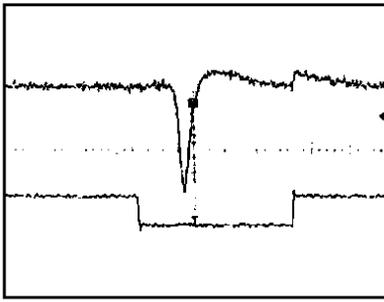
Fig. 10 Laser pulse waveform at the pulse repetition rate of 10kHz (500ns/div) and signal of voltage pulse
