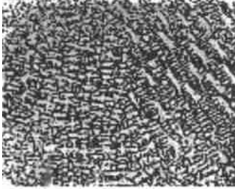
Fig. 2 Structure of laser cladding coating, Co-base alloy, corroding in aqua regia, 320 \times
