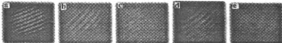
Fig. 5 Interferograms of damage process detected by the optimum Nomarski interferometer
