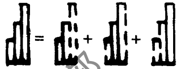
Fig. 2 Equivalence of binary gratings to Ronchi grating with different phase and position
