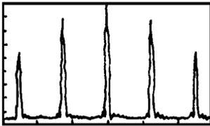
Fig. 2 The measured grating diffraction pattern when  $N_0$  (light intensity of Gaussian white noise) =  $A_0^2$  (power of inside laser intensity)
