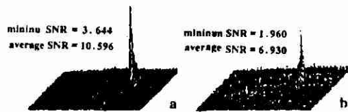
Fig.7 a, b, the maximum and minimum optical correlation S/N of SDF 3 and its training images
