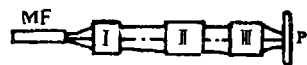
Fig. 1 The schematic diagram of focusing optical system MF - multimode optical fiber; P - marked workpiece; I - quasi-focusing optical system; II - enlarging and aligning optical system; III - focussing optical system
