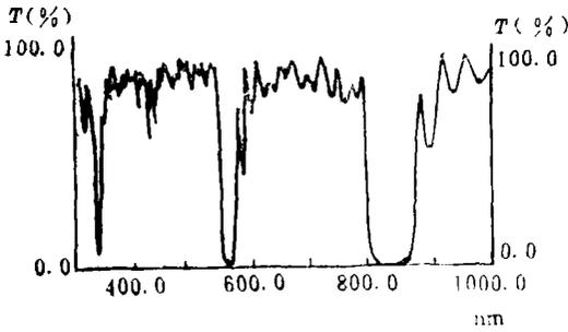
Fig. 5 Practical transmissivity curves of coated elements
