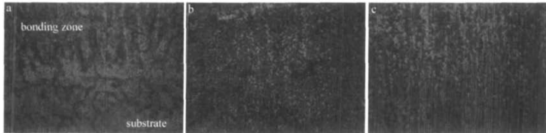
Fig 1 Microstructure of the laser cladding layer on pure aluminum surface (600 \times ) a—bonding interface b—middle interface c—upper interface
