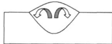
Fig 3 Schematic diagram of the flowing of the melting pool
