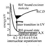
Fig 1 Potential curve diagram of exciner
