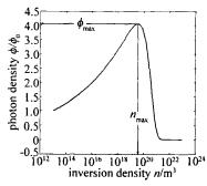
Fig 3 Photon density as a function of the inversion density
