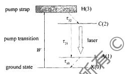
Fig 2 C→A transition exciner four level diagram
