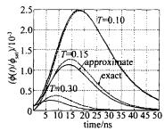
Fig. 4 Normalized intracavity photon density as a function of time for the different mirror transmissions
