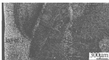
Fig. 4 Cross sectional microstructure of laser deposited nickel-based alloy coating
